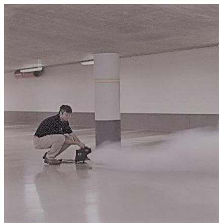
Figure 1 - A live smoke test is a good way of demonstrating the system performance
